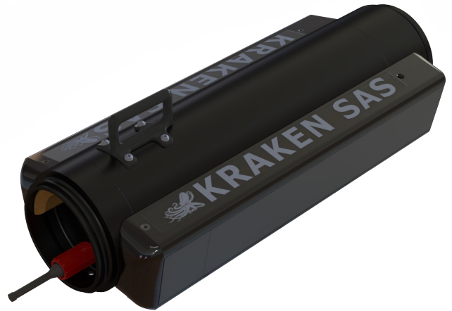
Above: Man-Portable SAS payload section designed for retrofit of small class vehicles.
