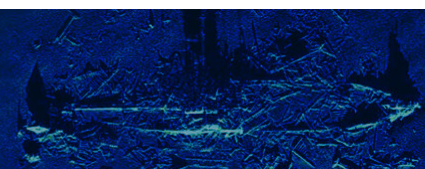
Visual representation of an actual buried UXO, with graphic overlay, located by the GeoLink. Previously undetected by magnetometry and sub-bottom profiler. SBI data imagery as seen in a real-time vertical slice.
