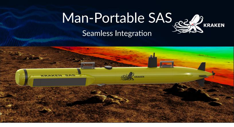
Kraken's MP-SAS payload is designed to retrofit existing man-portable UUVs and deliver full-swath, high-resolution Synthetic Aperture Sonar data from small vehicle platforms. Ideal for MCM/UXO/IPOE missions, the modular payload section can be added or removed in-field, allowing operators to keep the vehicles' OEM shipping containers.
