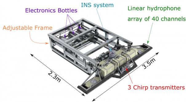
Fig. 1. Diagram of the Sub-Bottom Imager™ (SBI)
