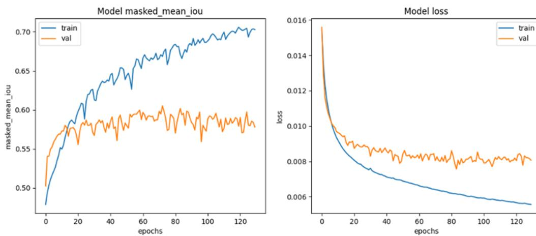
Fig. 5. Mean IoU and loss for model trained on multi-class masks using artificial classes and sigmoid corrected imagery.
