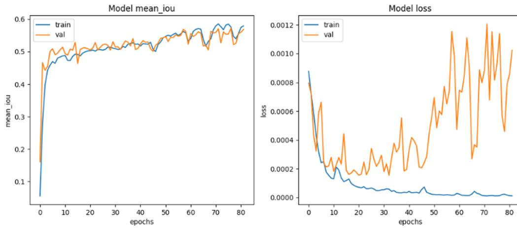
Fig. 3. Mean IoU and loss for model trained on binary masks without sigmoid correction to the imagery.
