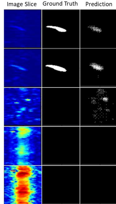
Fig. 6. Examples of model predictions; left column contains the image slices, the middle column represents the ground truth label, and the right column represents the 3-D U-Net prediction. In the ground truth and predictions white indicates target and black is background.
