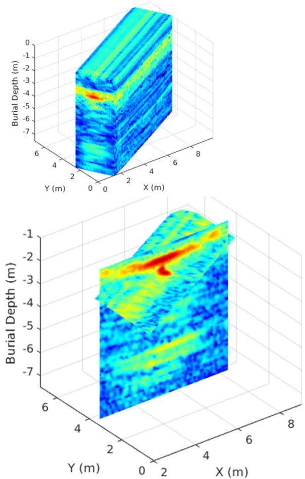
Fig. 2. Top: Rendering of a SBI seabed volumetric image used to train the 3-D U-Net model. Bottom: 2-D slices along the y and z (depth) axis to show target anomaly located inside the volumetric image above.
