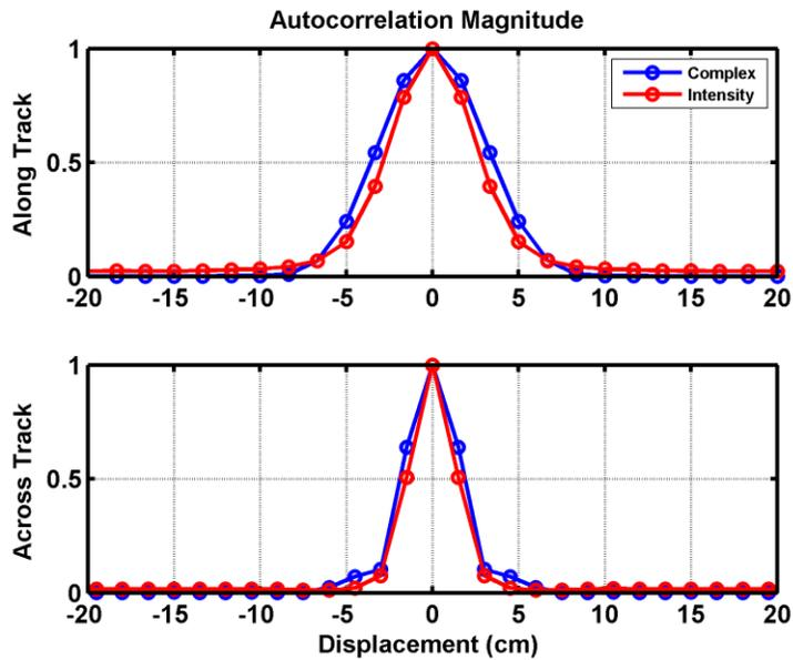
Figure 2: Along track and across track autocorrelation of complex SAS image and its intensity.
