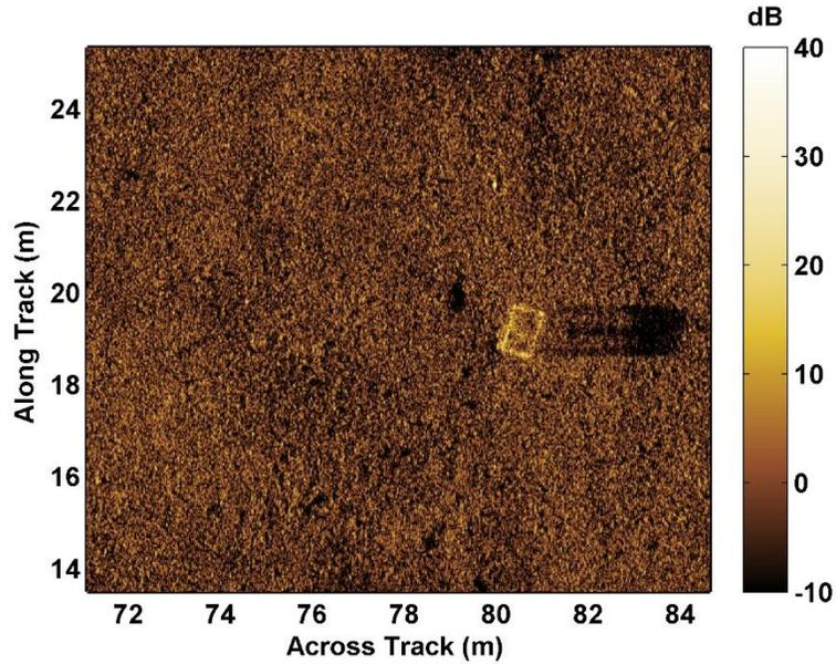
Figure 1: SAS image of cube target and a relatively featureless surrounding seabed.
