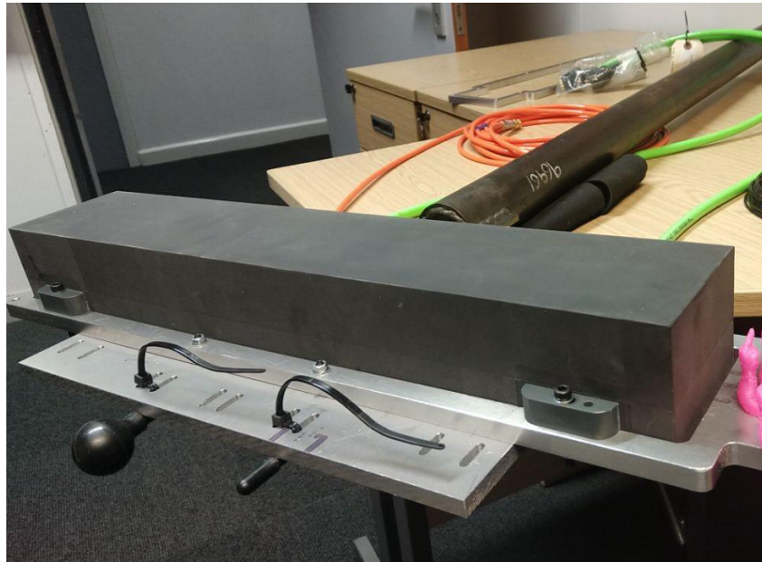
Figure 1: Prototype ultra-wideband receiver array (4–200 kHz).
