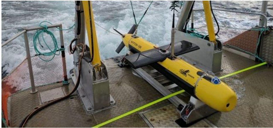
Figure 1: KATFISH actively controlled towfish with AquaPix ® MINSAS side-looking sonar.
